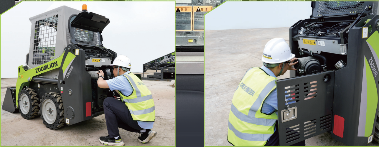
Large upper cover tipping angle for easy maintenance Oversized cab for easy inspection
